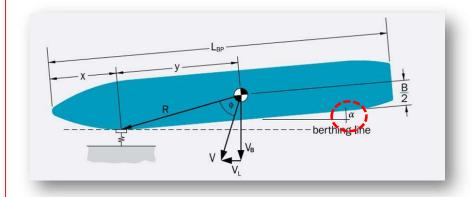
Berthing angle is a function of vessel size:
